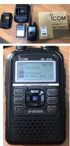
ICOM ID-31A D-STAR/FM UHF handheld transceiver. UHF only. Up to 5 watts output. Built in
