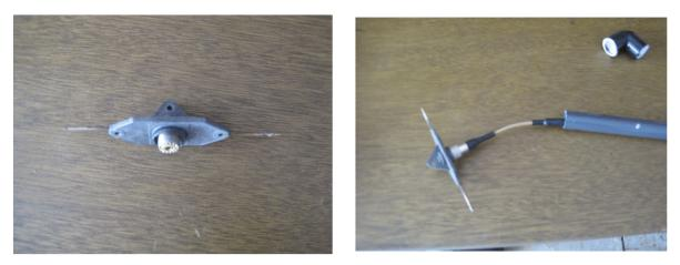
I attached my RF Choke Balun to my dipole center. (I dont use a traditional W2AU type balun with the fear that 1500 watts could fry it! The Coax Choke Balun uses 60 small common mode chokes around coax.) Use super glue or PVC cement to attach the dipole center to the 12 inch pipe.
